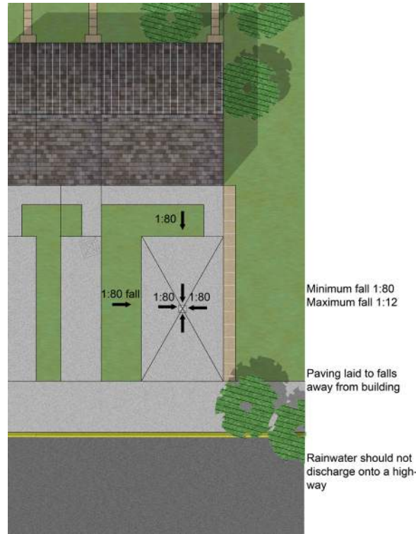
Figure 2: Drive and pathway drainage
