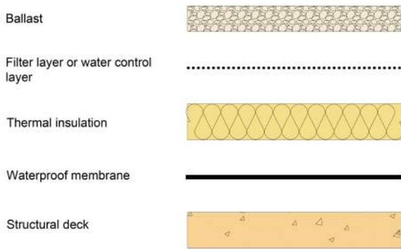
Figure 2: Inverted warm roof (section)
