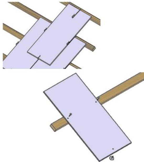
Figure 13: Fixing slates
