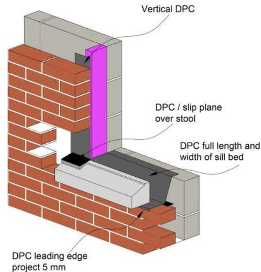
Figure 11: Stone sill with insulated cavity closer
