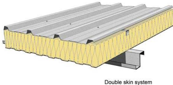
Figure 1: Typical metal double skin insulated roof
