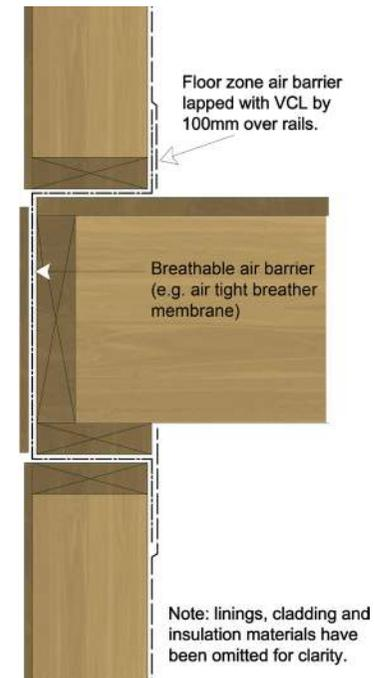
Figure 12: Typical floor zone air tightness detail
