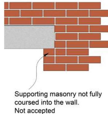
Figure 14: Incorrect method of brick bond around lintels
