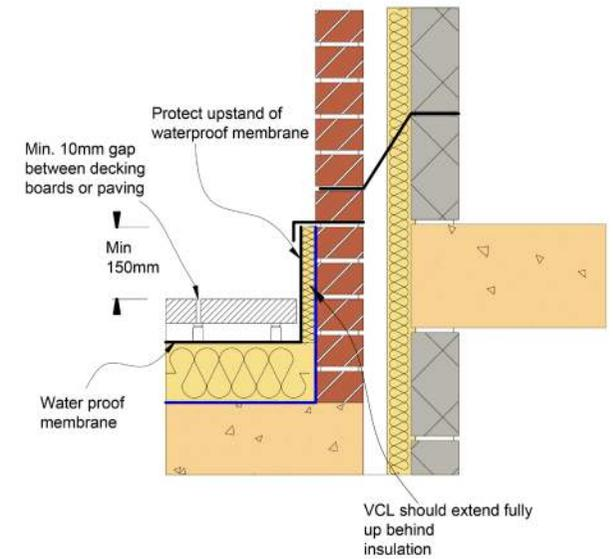
Figure 7: Details - Principles – Upstands to decking and paving finishes, (e.g. balcony parapet)
