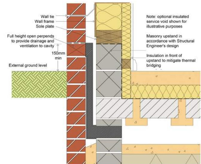
Figure 8: Kerb upstand detail to allow level threshold
