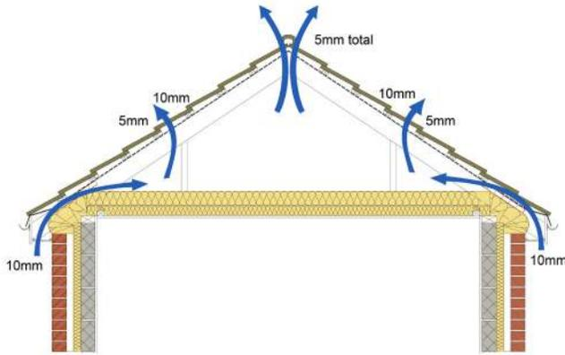
Figure 4: Duo-pitch roof with fire break walls
