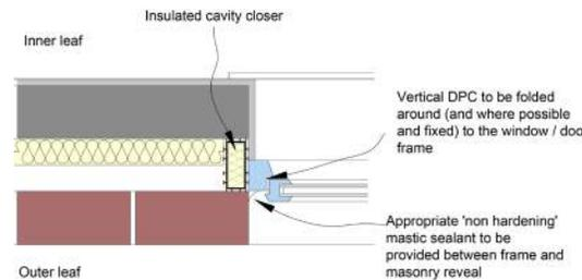
**Figure 7: Typical window reveal detail (normal exposure)**
