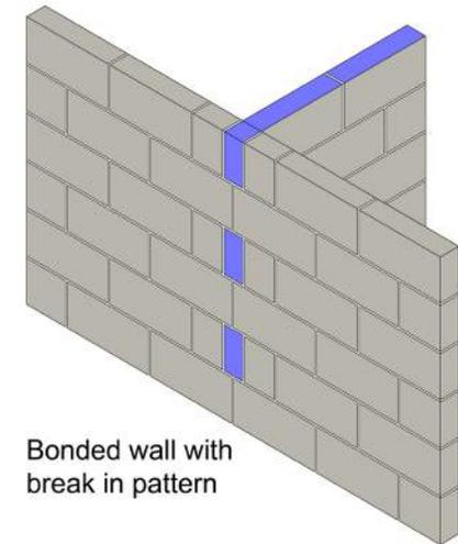
Bonded wall with break in pattern
