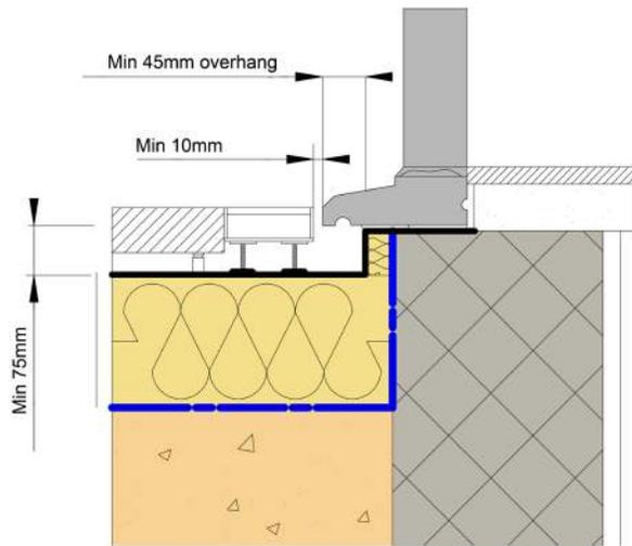
Figure 5: Details Principles – Upstand at door access
