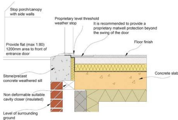
**Figure 3: Typical level threshold with canopy protection**
