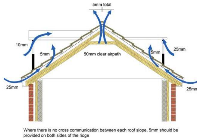
Figure 7: Pitched roof with pitched and flat dormers
