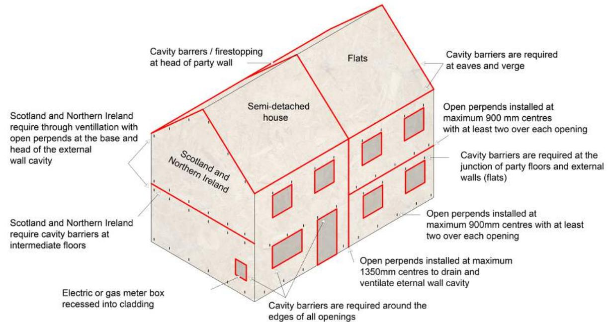
Figure 14: Locations of cavity barriers and open perpend
