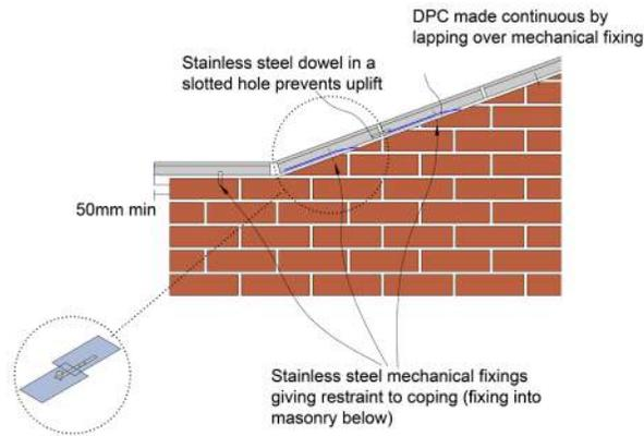
Figure 23: Fixing of copings to sloping parapets
