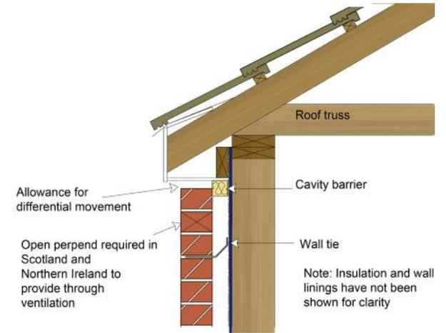
Figure 21: Differential movement at eaves
