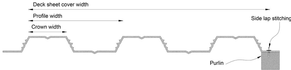
**Figure 9: Profiled metal decks - critical dimensions**
