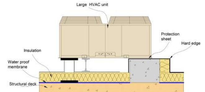
Figure 8: Detail – principles – plant support
