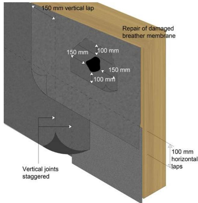
Figure 13: Lapping and repair of breather membrane
