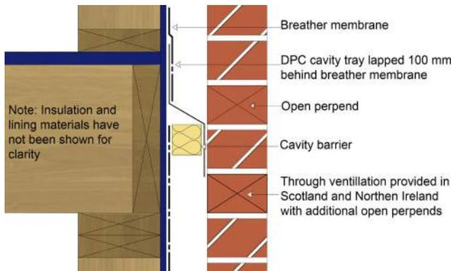
**Figure 15: Cavity tray above horizontal cavity barrier**
