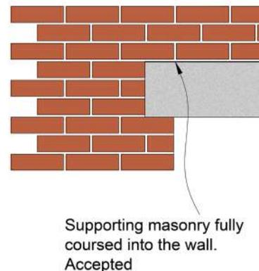
Figure 15: Correct method of brick bond around lintels
