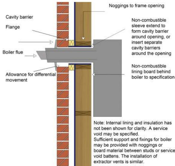
Figure 24: Differential movement at service penetration
