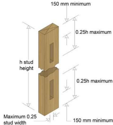
Drilling on centre line only. Hole diameters not greater than 0.25 stud width and hole centres not closer than  $4d$  ( $d$  = hole diameter)
