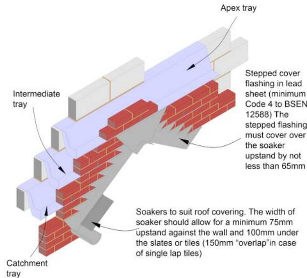
Figure 20: Stepped cavity at roof / wall abutments
