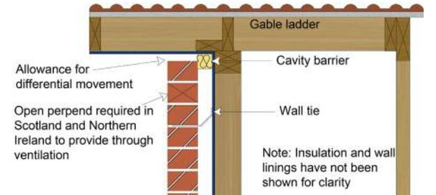
Figure 22: Differential movement at verge
