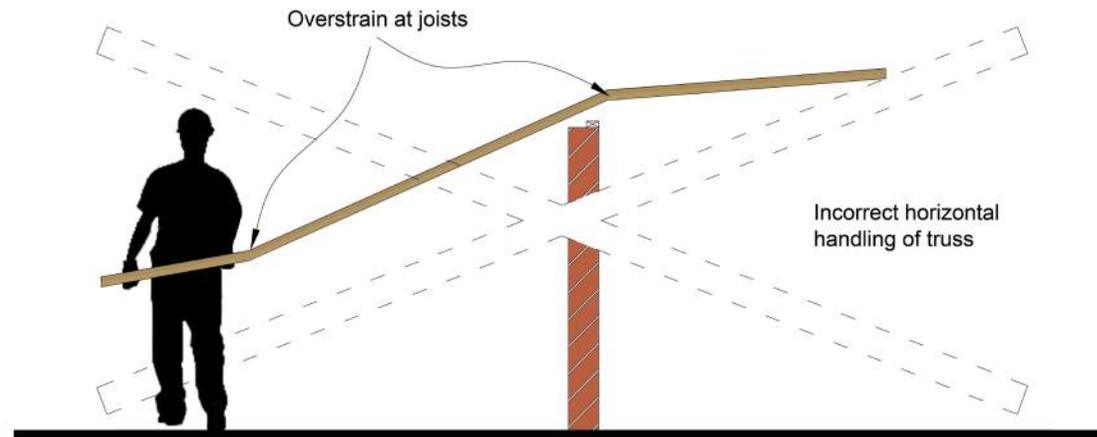
Figure 5: Avoid bending or see-sawing of trusses
