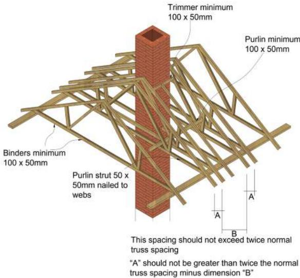
Figure 8: Roof trusses trimming around a chimney
