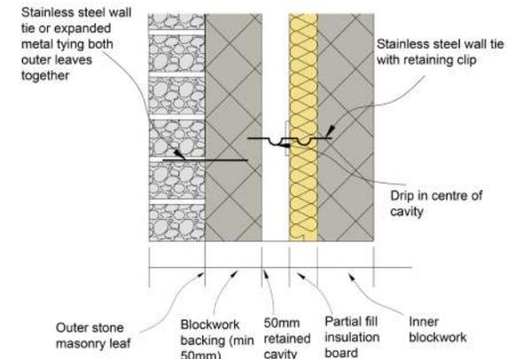
Figure 24: Masonry cavity wall with stone outer leaf
