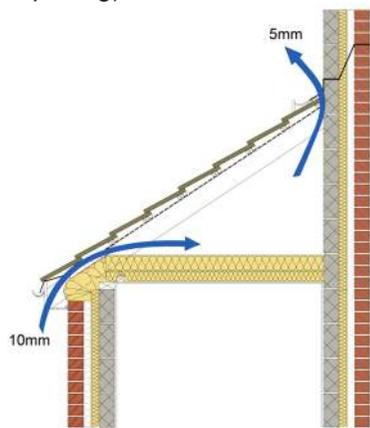
Figure 1: Mono-pitch / lean-to roof
