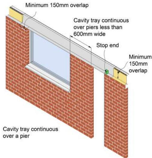
Figure 17: Continuous cavity tray over two openings and a small pier
