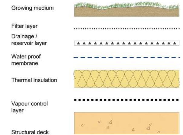
Figure 2: Intensive green roof - inverted warm roof (section)
