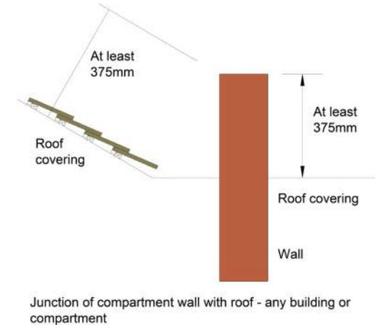
Figure 13: Typical fire stopping details
