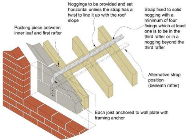
Figure 5: Lateral restraint strap to gable wall
