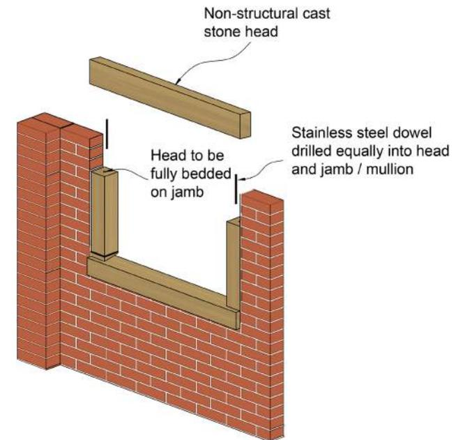
Figure 26: Joining stone jambs to sills and head
