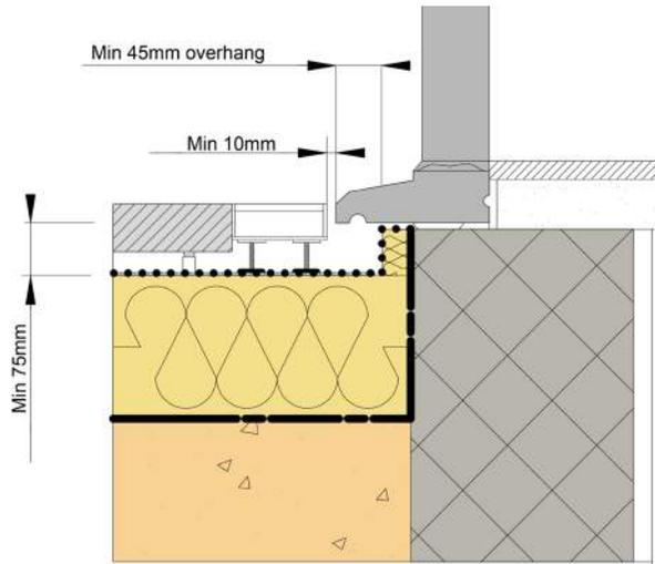
Figure 6: Details - Principles – Upstand at door access
