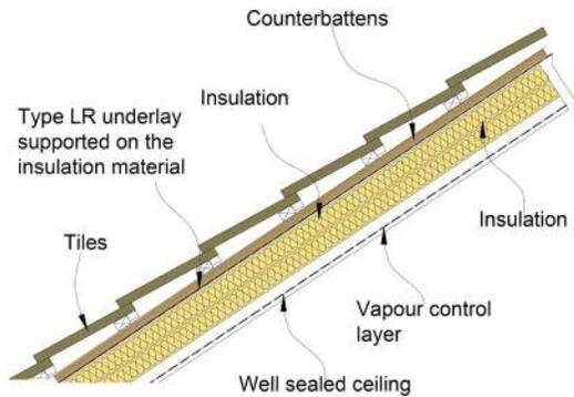
Figure 9: Warm roof construction (vapour breathable underlay)
