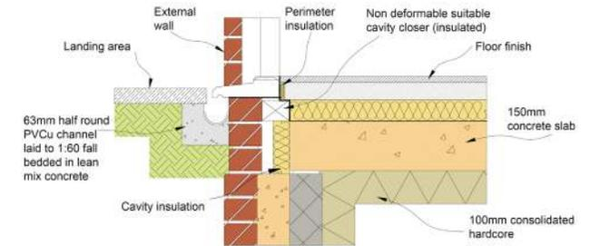
Figure 2: Typical level threshold suspended concrete slab
