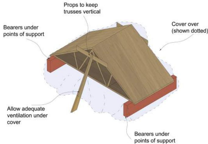
Figure 2: Site storage of trusses
