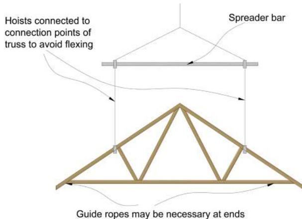
Figure 6: Mechanical lifting
